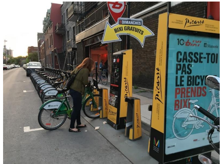
Example of a docked (station Based) bike share system in Montreal, Quebec. Users can access a bicycle at a physical docking station by unlocking the bike using a membership card, cell phone, credit card or other payment methods. Docking stations are distributed through a network within a designated service area. A bicycle trip both starts and ends a docking station.
