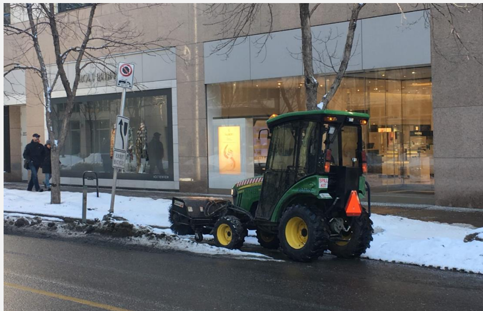
Example of a John Deere tractor from the City of Calgary that is clearing snow in a protected bike lane. This tractor has different attachments (brush, bucket, sprayer on the back) that can be used to clear snow, leaves, and other debris.
