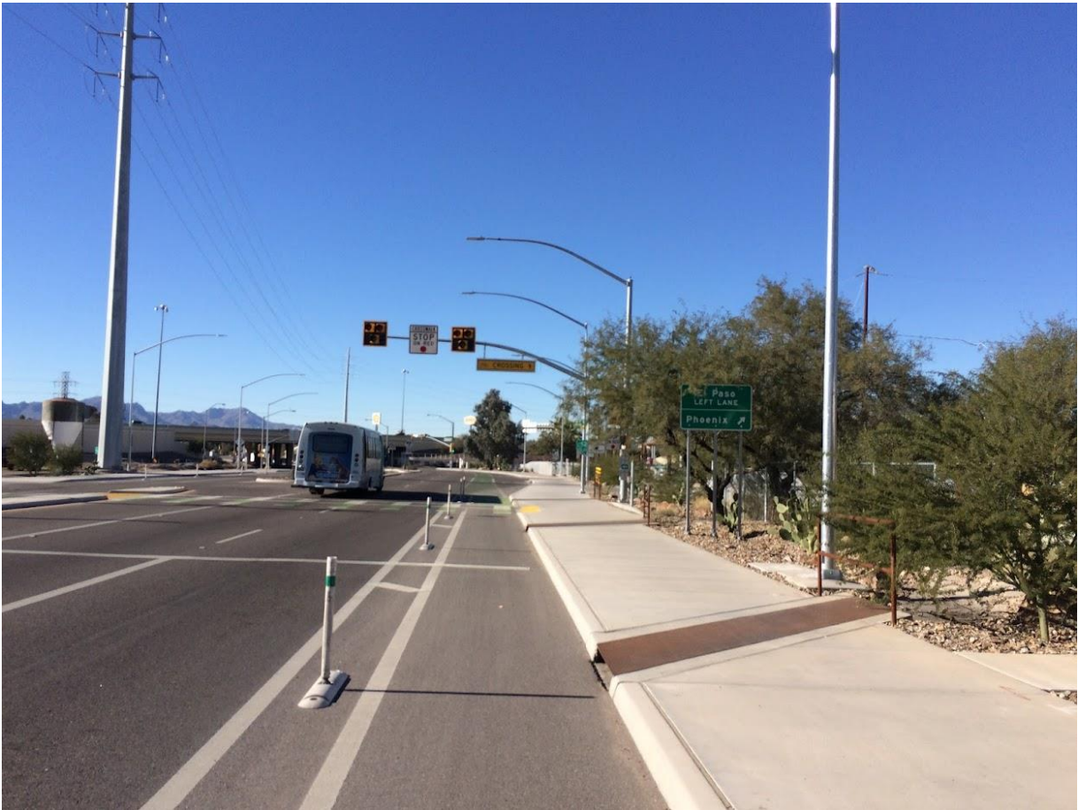
Example of a quick-build cycling facility in Tucson, AZ that has delineator posts as the separation material. This is the type of facility envisioned on Tillicum Road / Lampson Street as part of the quick-build network.
