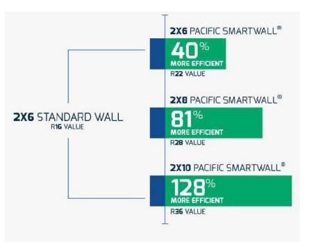
Pacific SmartWall® is a prefabricated wall system that simplifies your build and offers significant advantages over other construction methods. Proven Increases in thermal efficiency and air tightness combined with increased indoor air quality, reduced sound transmission and shorter framing timesthat's the Pacific SmartWall® Advantage.
