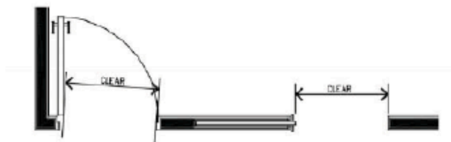
FIGURE 1 – CLEAR OPENING MEASUREMENT FROM DOORS
