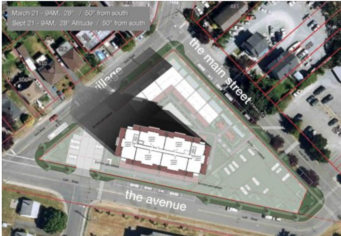
Morning shadows studies at 9AM March 21st, and September 21st, demonstrating shadows cast from both the fifth and sixth floor levels. These shadows approach but do not impose on residential properties.
