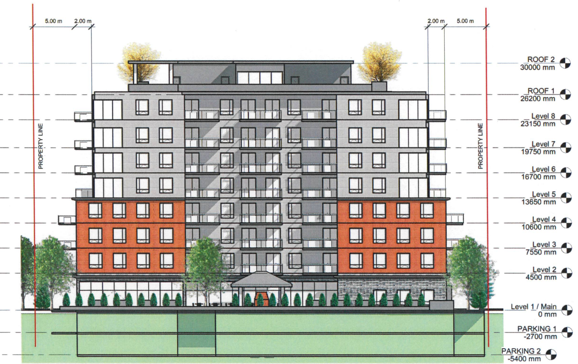
② South 1 : 200 BALCONIES ARE TO BE RESOLVED - SHOWN TO ILLUSTRATE PROPOSED SETBACKS ONLY
