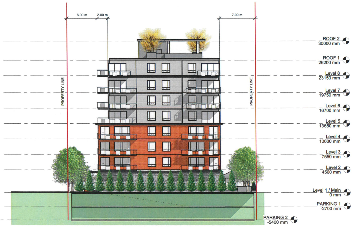
④ West 1 : 200 BALCONIES ARE TO BE RESOLVED - SHOWN TO ILLUSTRATE PROPOSED SETBACKS ONLY
