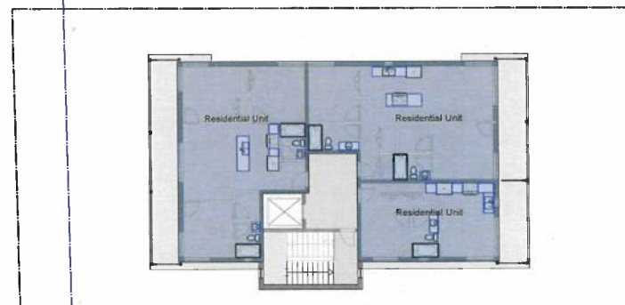
3 Typical Floor Area x 5 (FAR Calculation) Scale: 1:200 Area: 207 m 2 x 5
