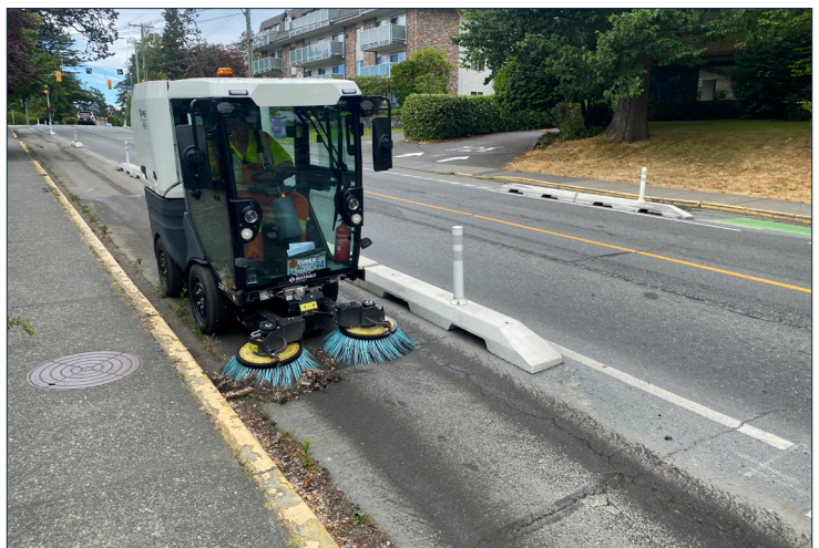
New street sweeper designed for bike lanes.
