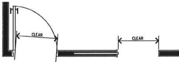
FIGURE 1 – CLEAR OPENING MEASUREMENT FROM DOORS
