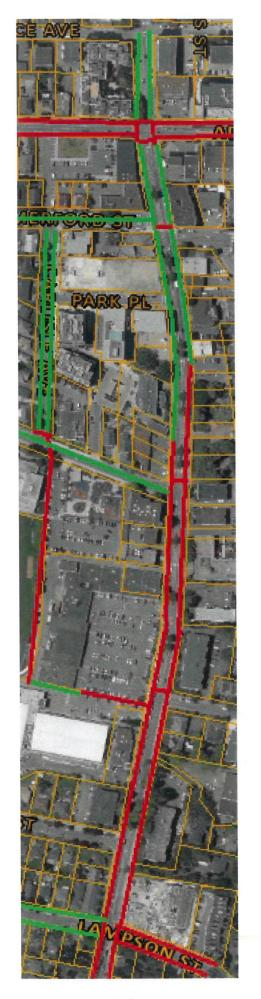
Archie Browning Protected Bike Lane with Buffer with Small Car Parallel Parking Stalls 9 Parking Stall Loss (18 Large Vehicle Stalls (20ft/6m) removed and 9 Small Vehicle Installed (16ft/5m)
