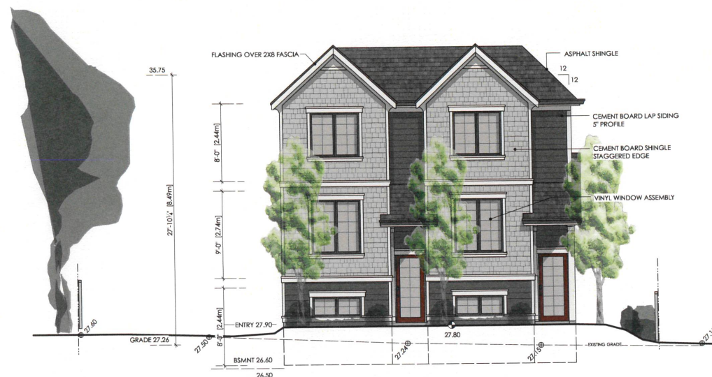
1 South Elevation, Facing Old Esquimalt Road Scale: 1:75
