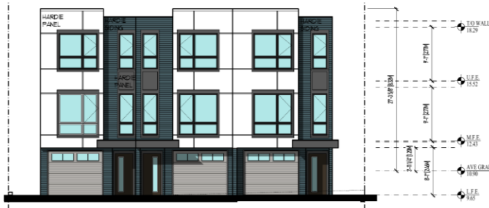
4 NORTH ELEVATION - LOT B A03 SCALE: 1/8"=1'-0"
